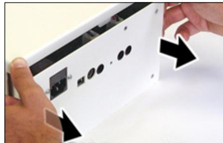
**5** Pull out the battery tray carefully. Note: The battery cables may catch on the sheet metal lip during removal.
