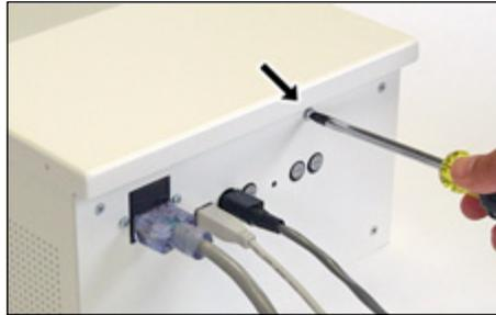
**1** Use the Phillips screwdriver to remove the two screws from the front of the enclosure. Then remove the screw (top center) from the back, as shown.
