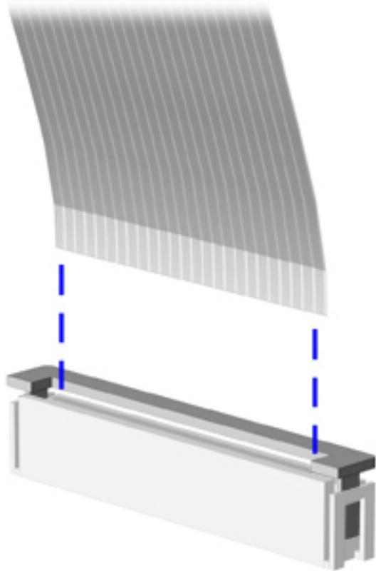
The computer uses a zero insertion force (ZIF) connector for the keyboard cable to the system board. To remove a cable from a ZIF connector, lift both corners of the ZIF connector and slide simultaneously with constant light force.
