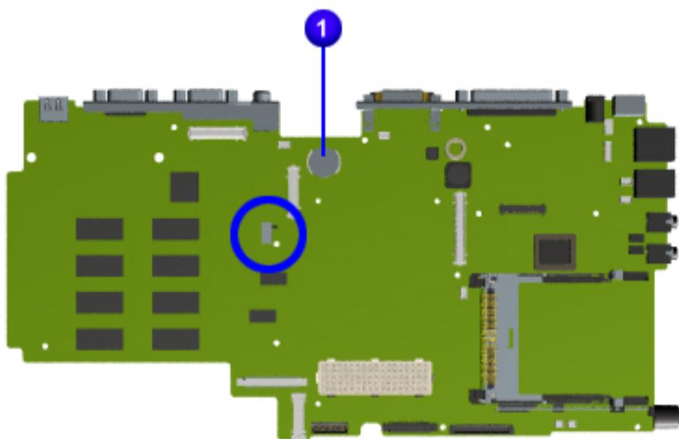
Clearing the power-on password requires removing all Setup attributes that are programmed in the CMOS. The **1** RTC battery is located on the system board directly forward of the fan.
