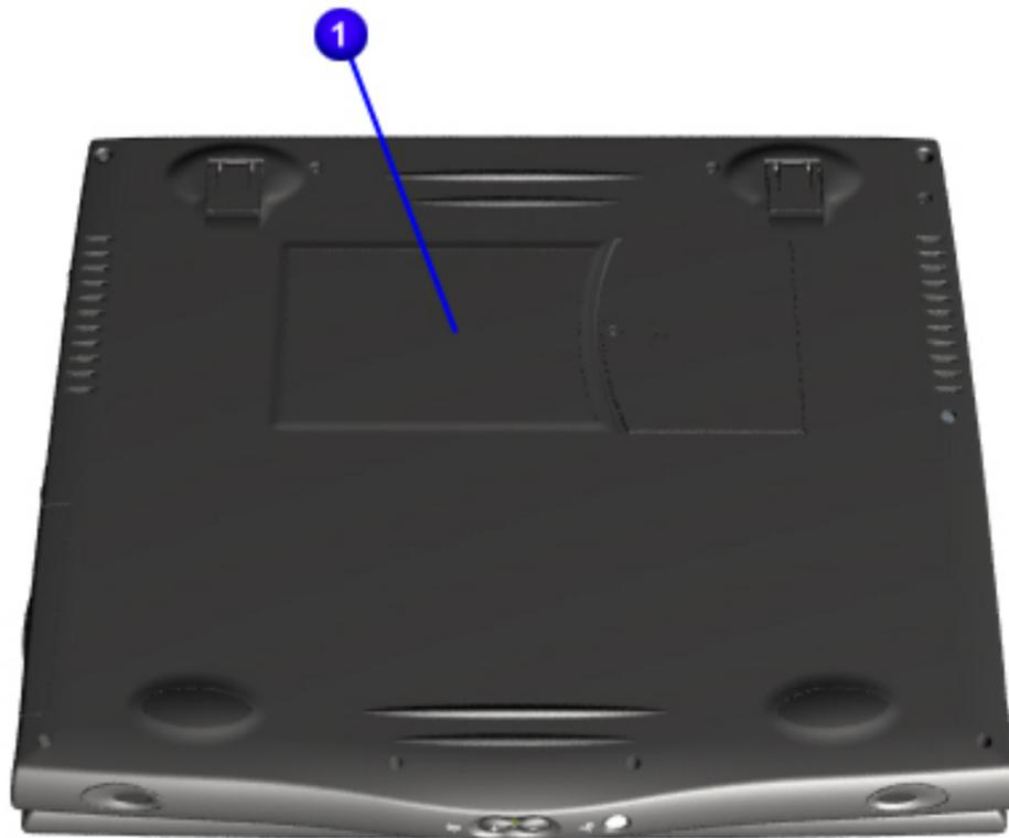
Report the computer serial number **1** to Compaq when requesting information or ordering spare parts. The serial number is located on the underside of the computer.
