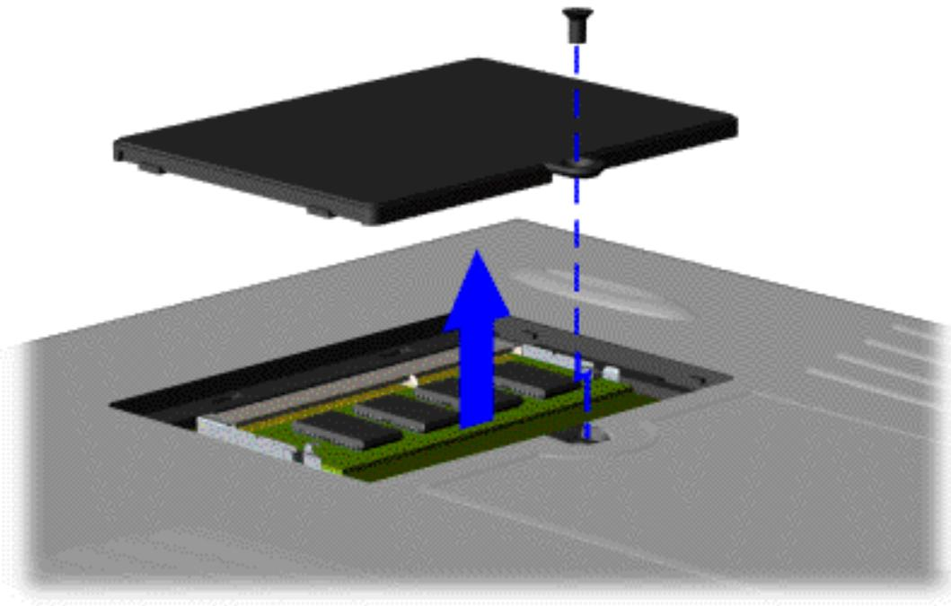
To remove the memory module, complete the following steps:
