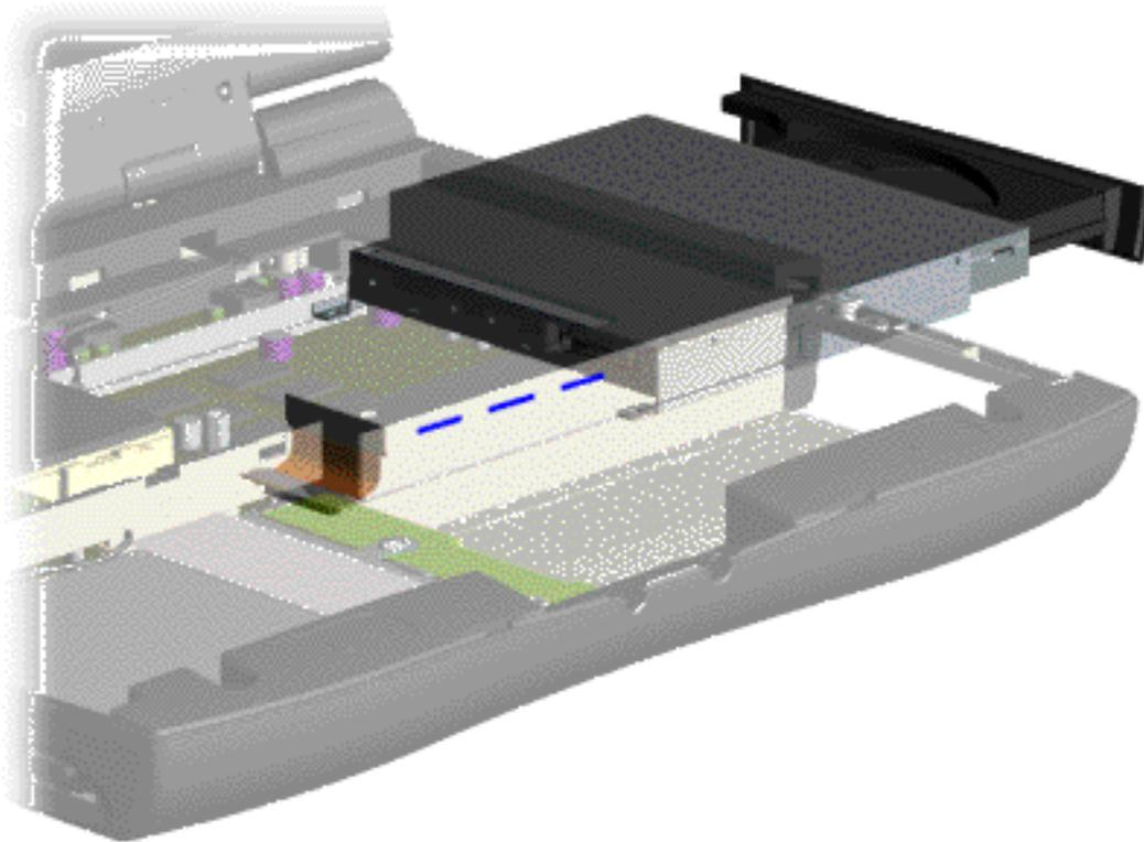
7. Disconnect the CD drive cable from the CD drive and remove the CD drive from the chassis.
