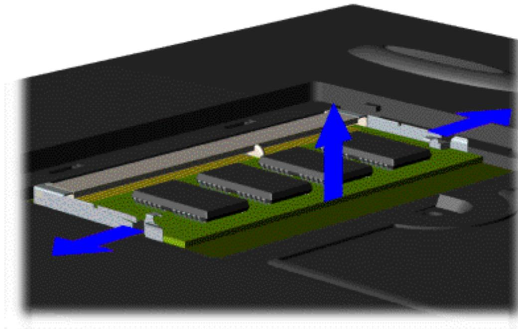
4. Pull side levers to release the memory module and unplug the memory module from the system board.
