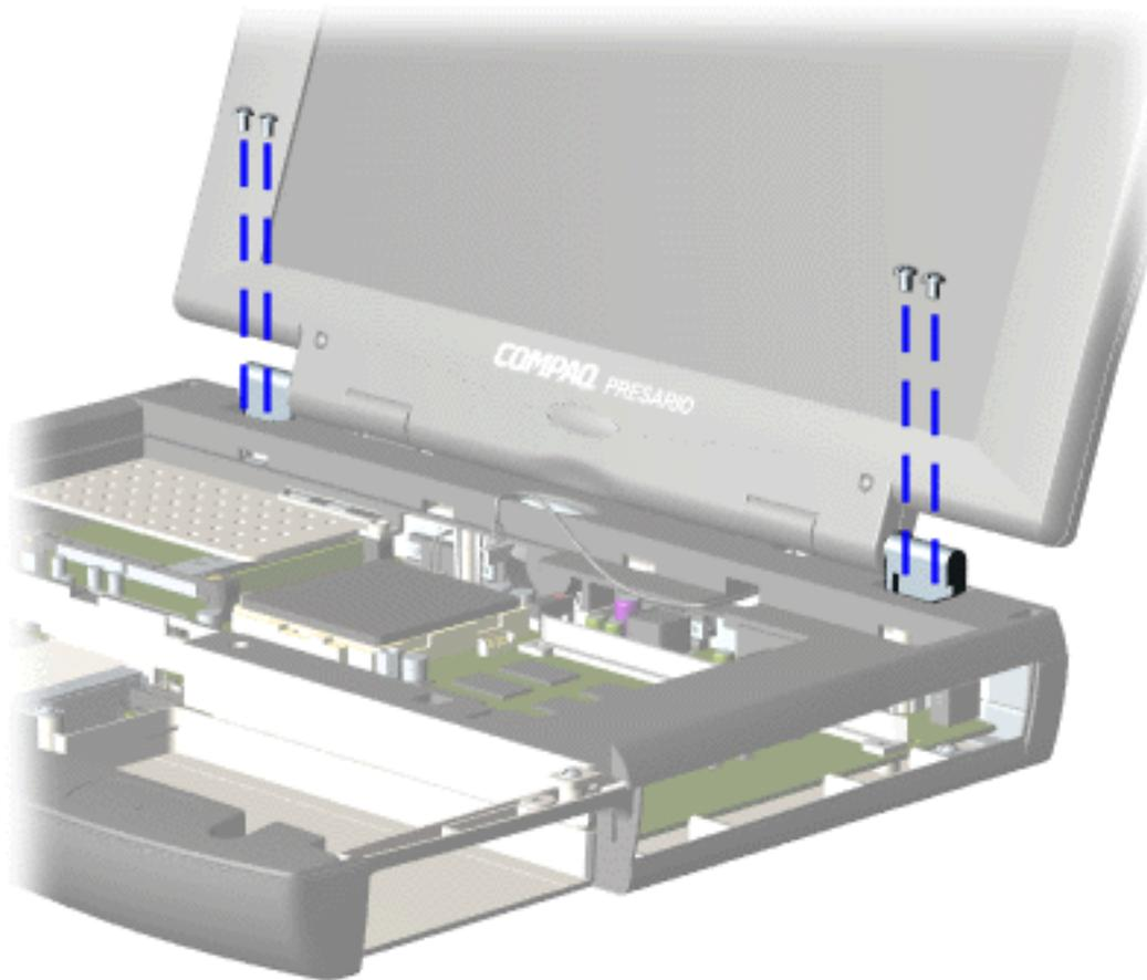
9. Support the back of the display panel assembly and remove two screws from each of the display panel hinges.
