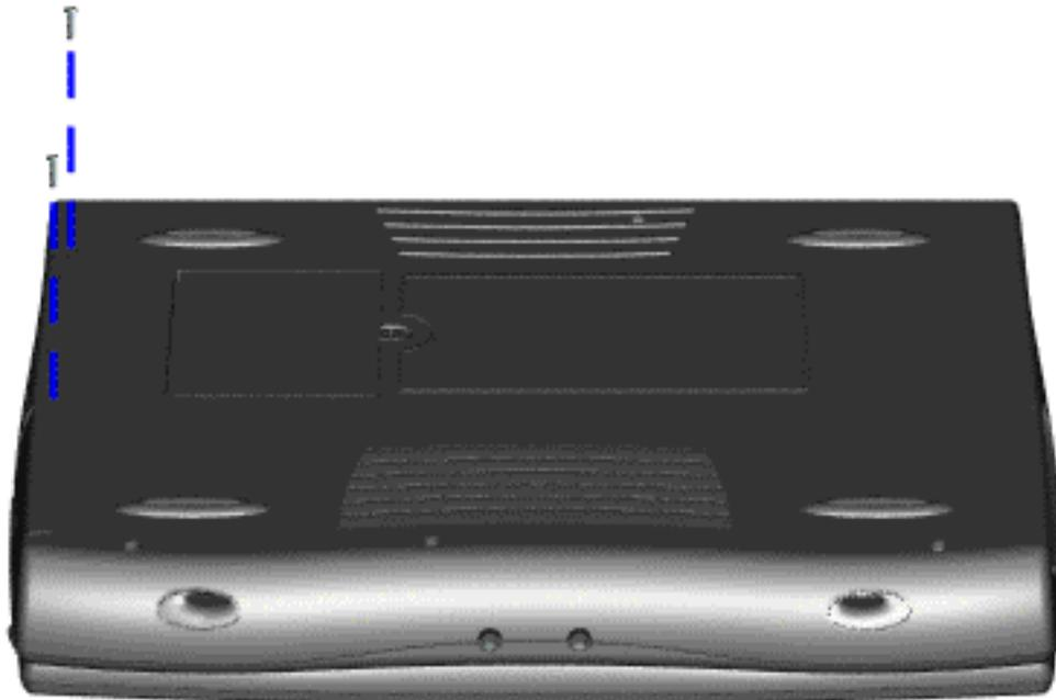
6. Remove the two screws on the bottom of the unit that secure the CD bracket to the system board.
