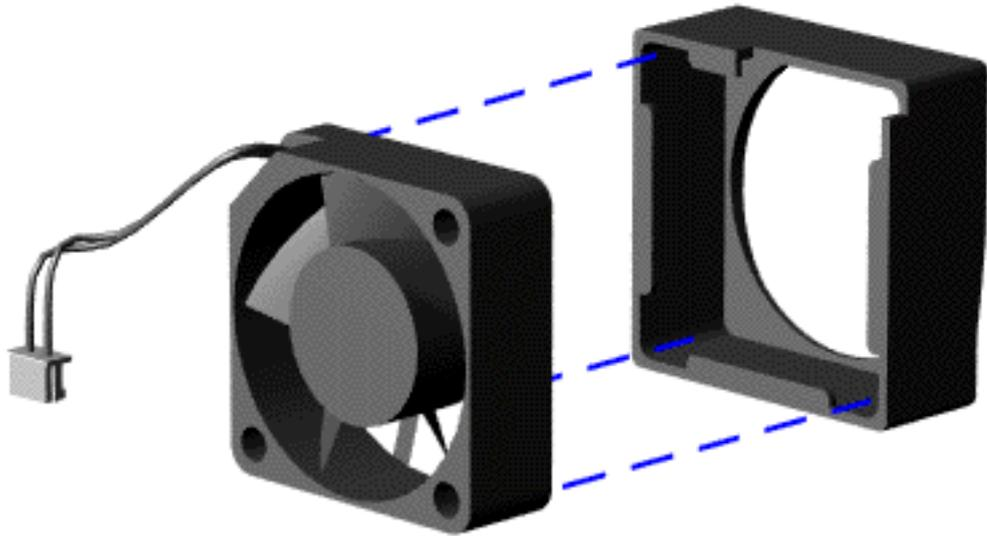
To remove the fan gasket, complete the following step:
