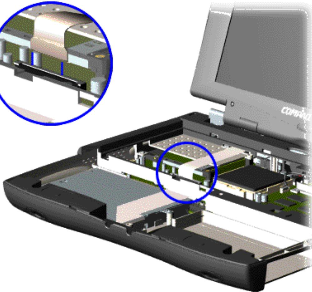
7. Disconnect the flex cable attached to the display panel assembly from the ZIF connector on the system board.
