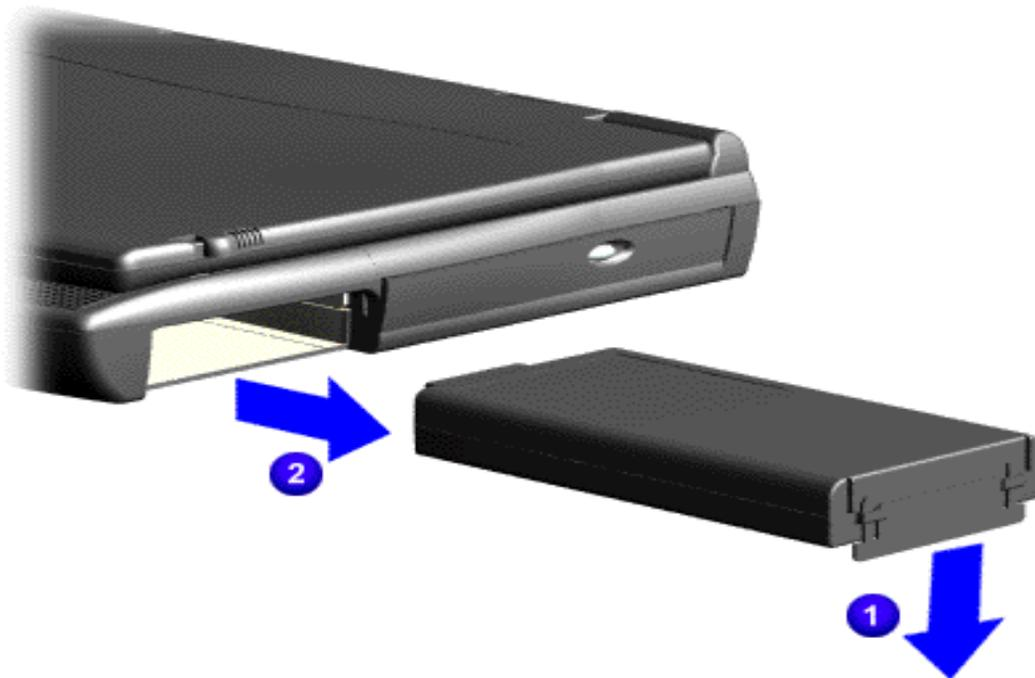
2. Pull forward on the battery pack tab **1** and remove the battery pack **2** from the chassis.
