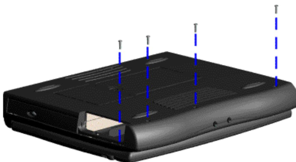
The palmrest cover with touch pad must be removed to gain access to any of the interior components of the computer, and it is the first component that has to be removed to gain access to the interior components.
