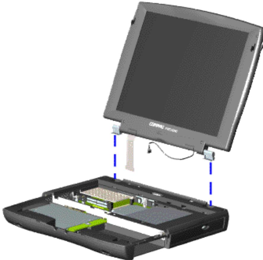
10. Gently pull the flex cable attached to the display panel assembly through the slot on the Upper CPU cover and remove the display panel assembly with flex and backlight cable attached.
