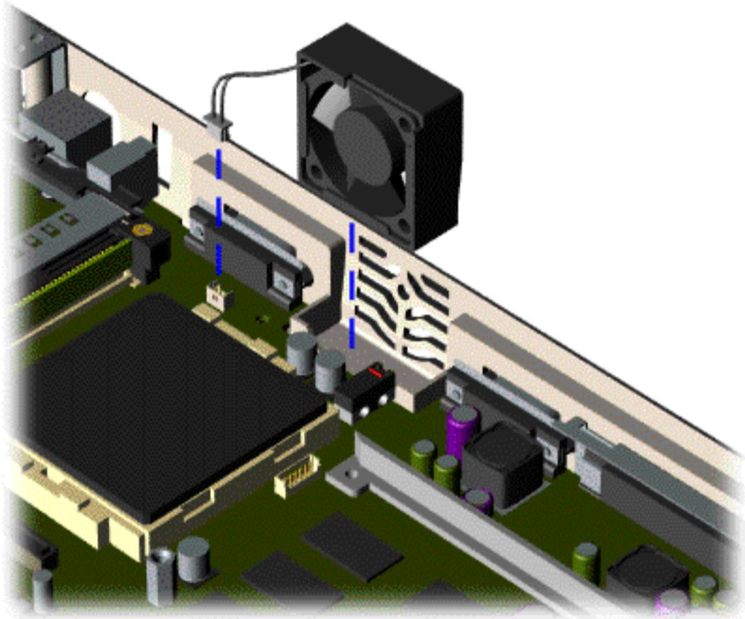
To remove the fan assembly, complete the following steps:
