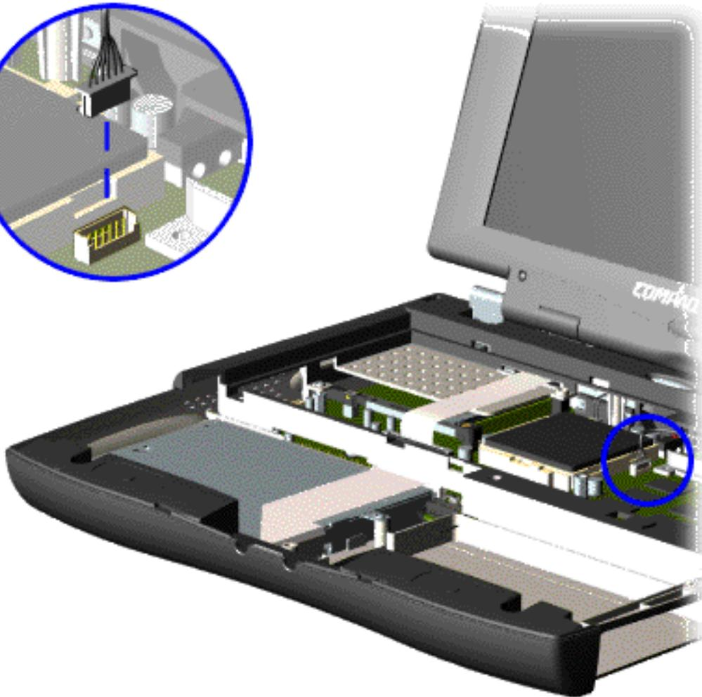
8. Disconnect the backlight cable attached to the display panel assembly from the connector on the system board.
