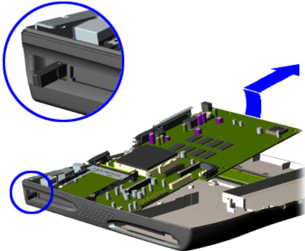
18. Pull the PCMCIA eject lever out (straight), lift up the right side of the system board and pull forward to remove the system board from the chassis.
