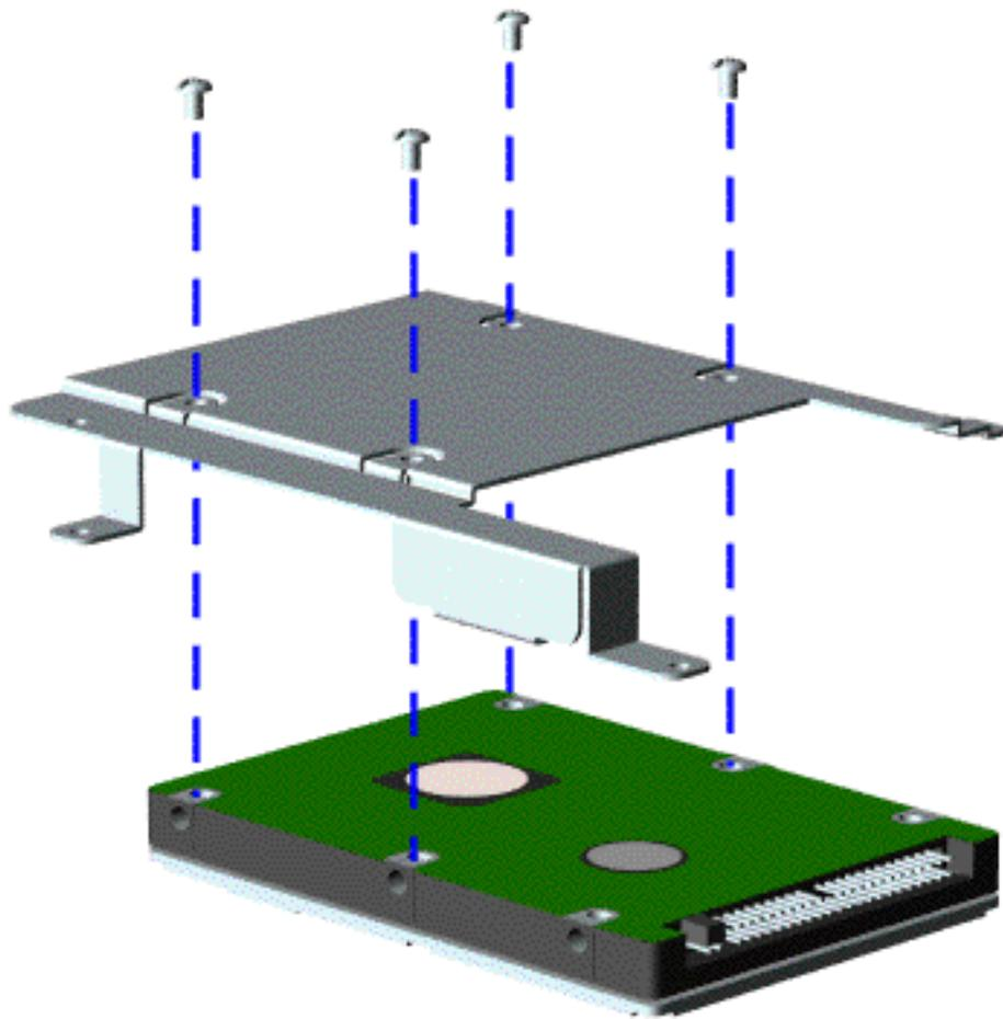
To remove the hard drive mounting bracket, remove four screws from the mounting bracket as shown in the illustration.
