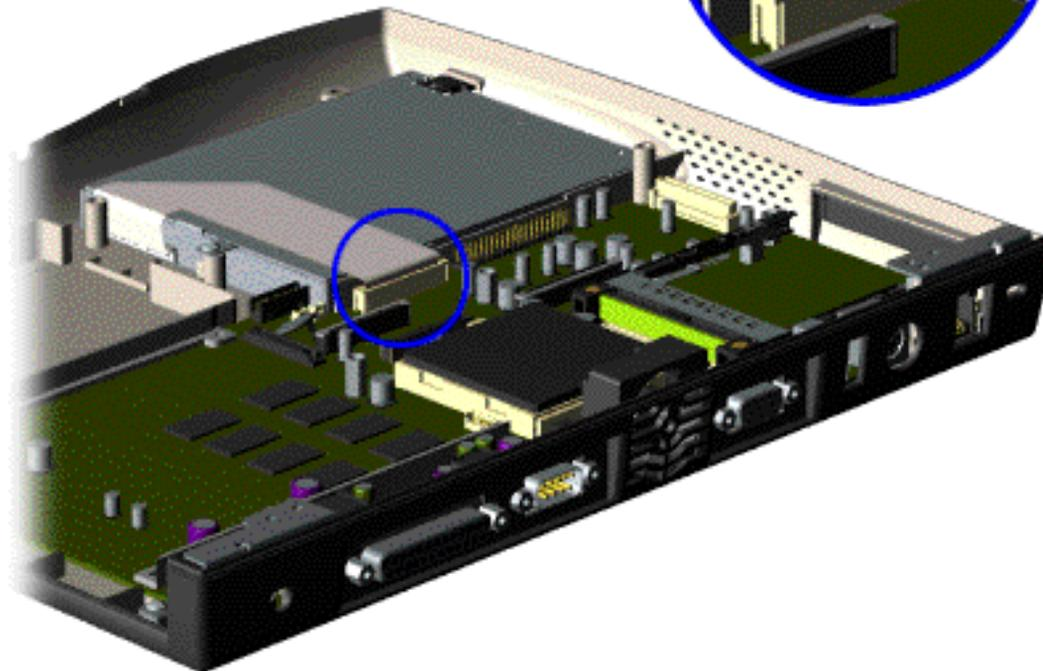
10. Disconnect the diskette drive data cable from the system board.
