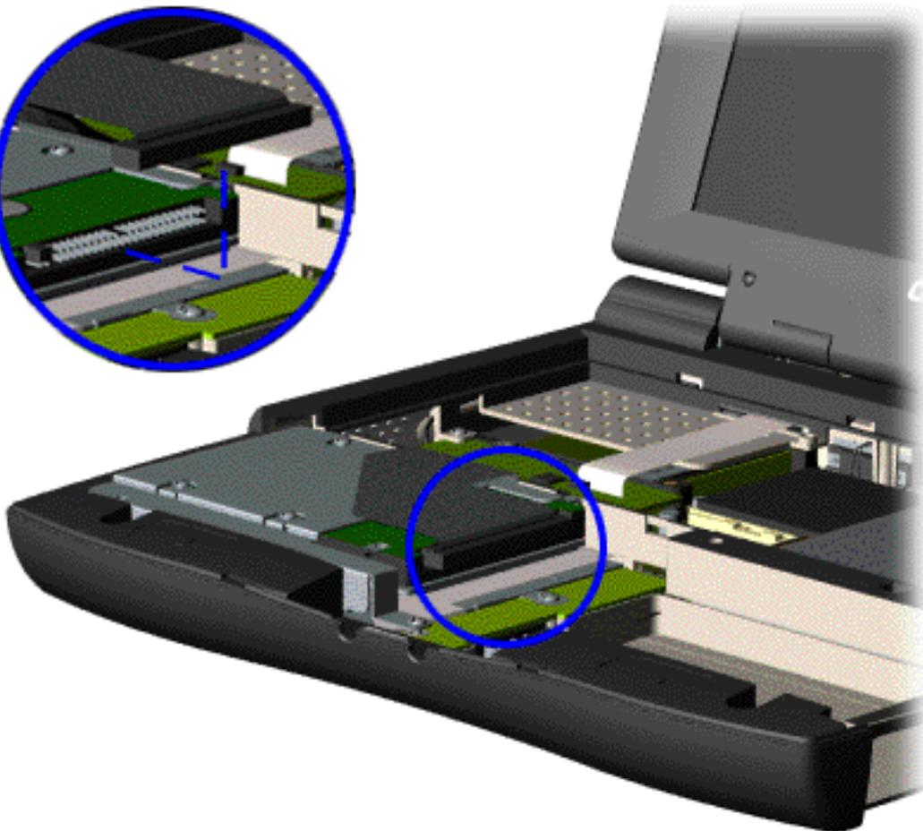
5. Disconnect the hard drive data cable from the hard drive and remove from the chassis.
