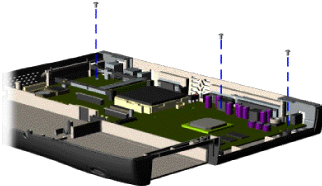
17. Remove three screws from the system board.
