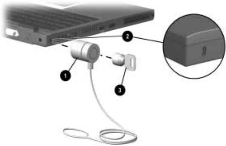
To remove the device, turn the locking device counterclockwise 90 degrees and remove the device from the slot.
