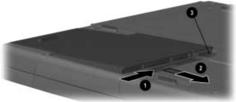
***Removing the battery pack***
