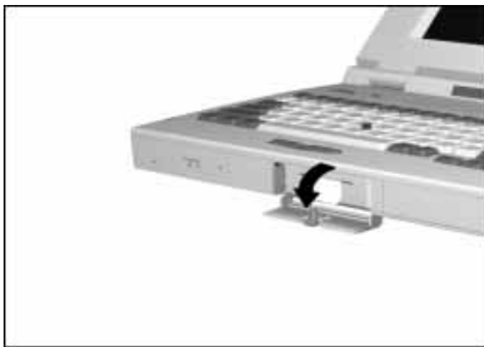
Opening the Hard Drive Door
