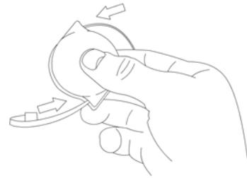
**STEP 3** - To retract the cable, push black button located on the bottom.
