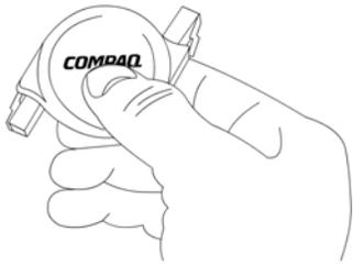
**STEP 1** - Hold your 6' Auto Retractable Phone Cable with one hand while gently pulling the modules outward.
