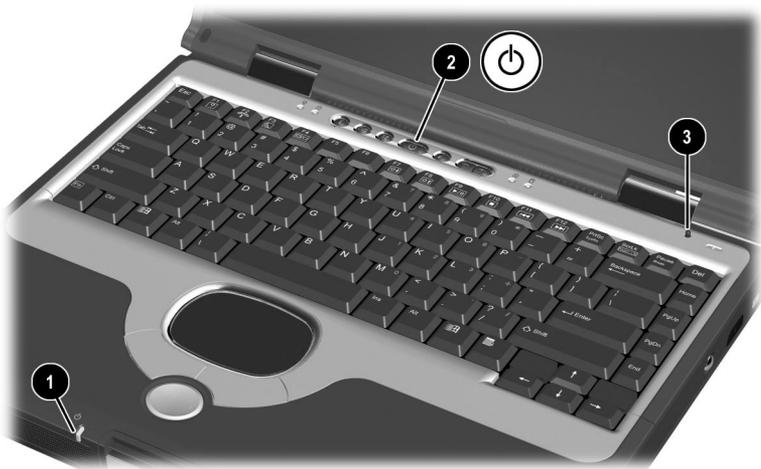
***Identifying the power/standby light, power button, and display switch***
