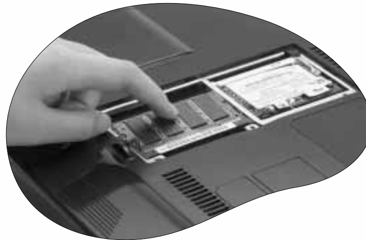
7. Gently push the free edge downwards until the module locks into place.
