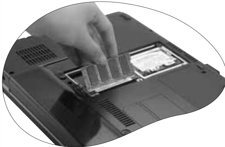
6. Align the memory module with the slot, and then insert it. When inserting, pay attention to the direction of the memory module.
