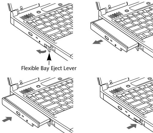
Figure 2-19 Removing/Installing a device in the Flexible Bay
