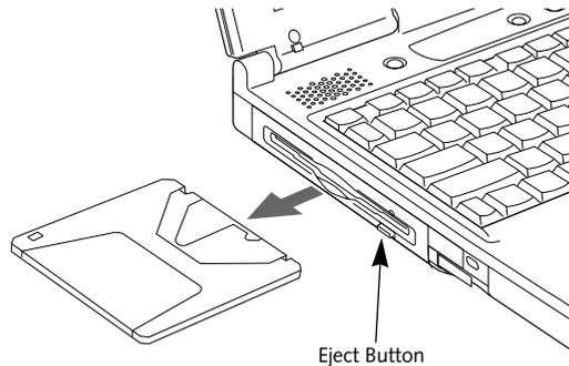
Figure 4-4 Loading/Ejecting a SuperDisk or 3.5" Floppy Disk
