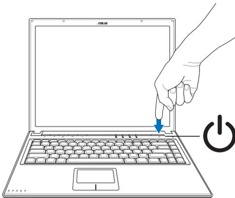
(2) Press the shutdown button
