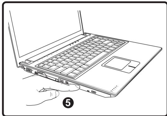
4. Slowly push the drive's tray back in. The drive will begin reading the table of contents (TOC) on the disc. When the drive stops, the disc is ready to be used.
