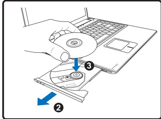
2. Gently pull on the drive's front panel and slide the tray completely out. Be careful not to touch the CD drive lens and other mechanisms. Make sure there are no obstructions that may get jammed under the drive's tray.
