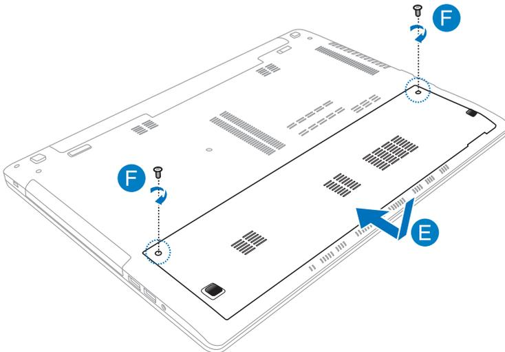
If you need to remove the installed RAM module from its slot, refer to the illustration below.
