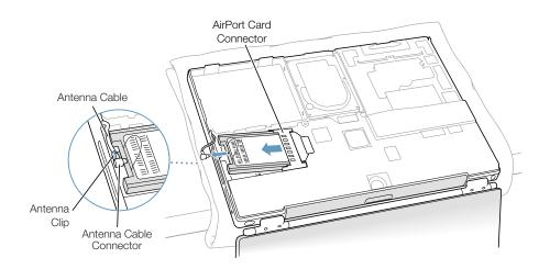
**Important:** If an AirPort Card is **not** being reinstalled right away, the antenna cable connector must be replaced into its holder (shown in step 4) and the loop of the antenna cable pulled up slightly and away from the edge of the computer case. This prevents the cable from interfering with the PC card slot, below, or getting pinched during reassembly.
