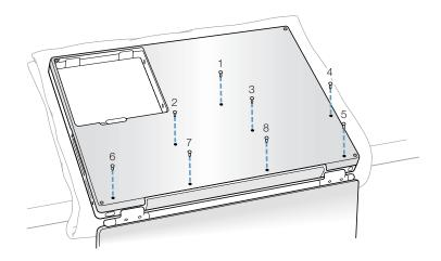
7. To remove the bottom case you will need to disengage it at the left and right sides, then carefully pivot it forward to release a retaining clip near the DVD drive slot, as follows.
