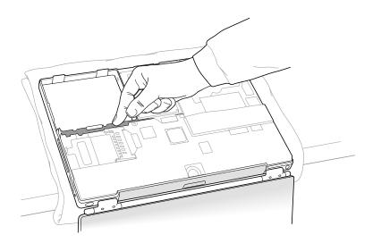
2. If removing an existing AirPort Card (if not, skip to step 3), pull back on the antenna clip to release the antenna connector and allow the card to rise up slightly, then pull the card from the AirPort connector.
