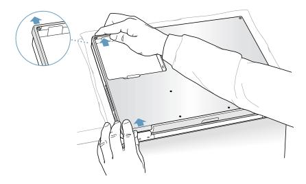
At the right side, again carefully slide the bottom case slightly up and away from you by pushing it just above the hinge of the display, and at the same time from within the battery compartment, pushing away from you at the right-most edge of the bottom case, until the right side releases.
