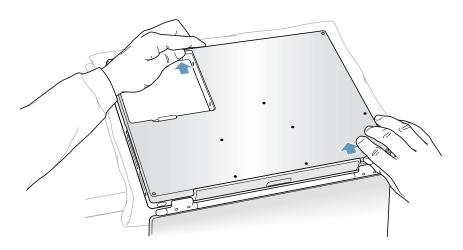
8. When both the left and right sides have released, carefully pull up on the bottom case at the edge that is closest to you and rotate it away from you, pivoting evenly over the front edge to release a retaining clip that is located near the DVD drive slot.
