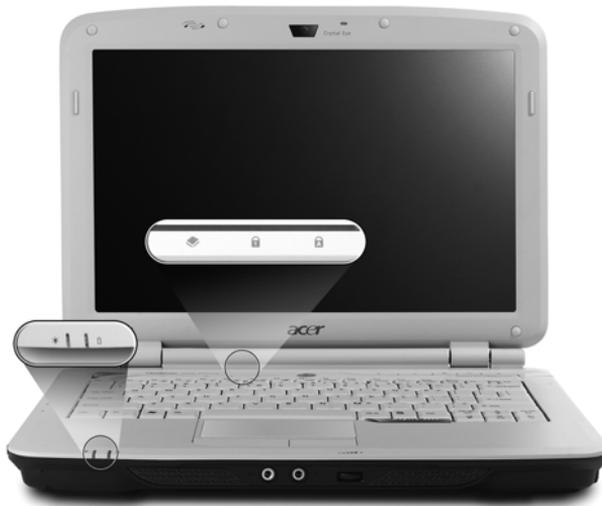
The front panel indicators are visible even when the computer cover is closed up.
