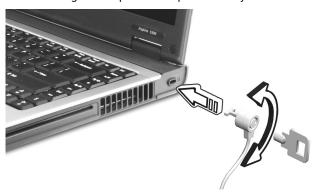
Wrap the computer security lock cable around an immovable object such as a table or handle of a locked drawer. Insert the lock into the notch and turn the key to secure the lock. Some keyless models are also available.
