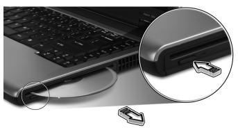
When the power is off, you can eject the drive tray by using the emergency eject hole (tray design drives only.)
