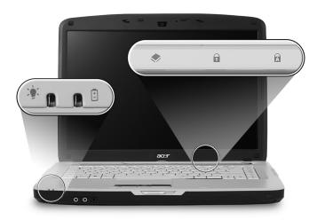
The front panel indicators are visible even when the computer cover is closed up.
