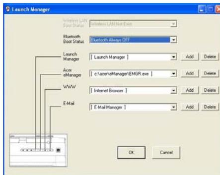
Launch Manager allows you to set the four easy-launch buttons located above the keyboard. **"Easy-launch buttons" on page 10** for the location of the easy-launch buttons.
