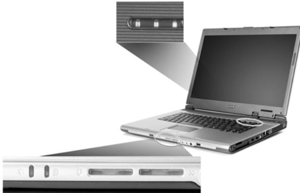
The power, battery and wireless communication status indicators are visible even when the LCD display is closed.
