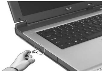
Insert a clip to the emergency eject hole to eject the optical drive tray when the computer is off.
