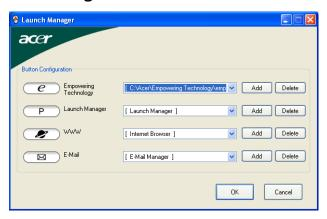
Launch Manager allows you to set the four easy-launch buttons located above the keyboard. "Easy-launch buttons" on page 22 for the location of the easy-launch buttons.
