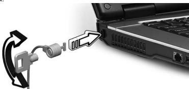
Wrap the computer security lock cable around an immovable object such as a table or handle of a locked drawer. Insert the lock into the notch and turn the key to secure the lock. Some keyless models are also available.
