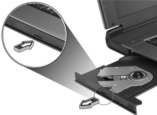
When the power is off, you can eject the drive tray by using the emergency eject hole.
