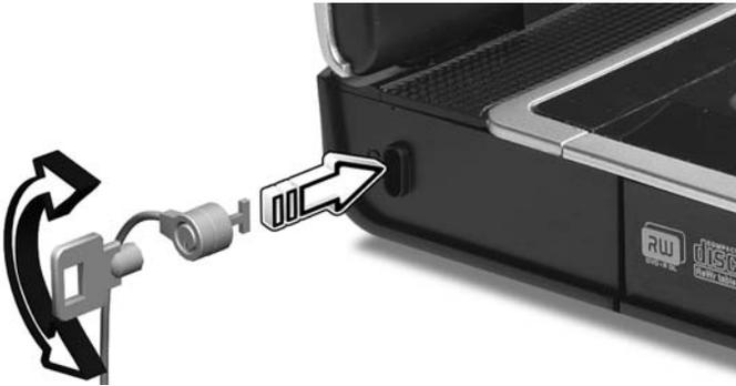
Wrap the computer security lock cable around an immovable object such as a table or handle of a locked drawer. Insert the lock into the notch and turn the key to secure the lock. Keyless models are also available.
