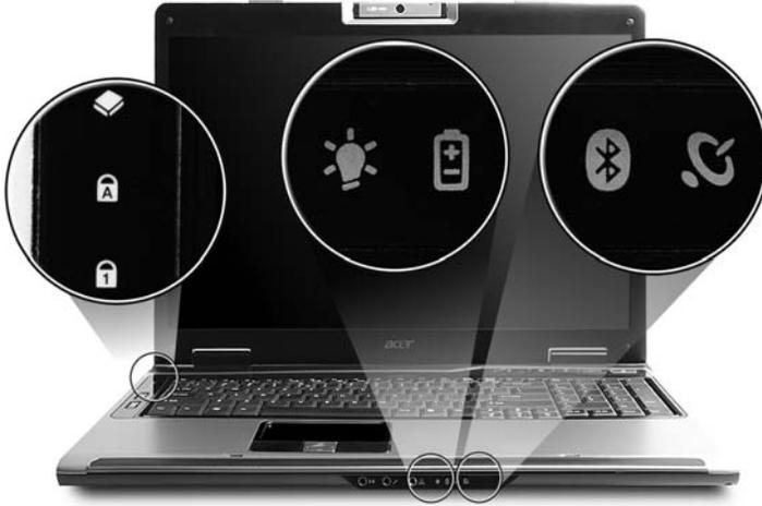
The front panel indicators are visible even when the computer cover is closed up.
