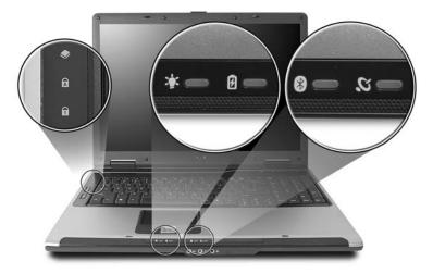
The front panel indicators are visible even when the computer cover is closed up.
