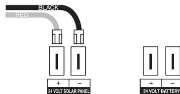
**IMPORTANT:** Improper installation of these wires will cause damage to the APeX controller or solar panel.
