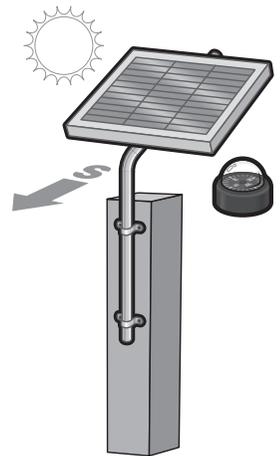
**IMPORTANT:** the solar panel must be positioned facing the path of the sun, due south and in an open area away from shade. It should receive at least 8 hours of direct sunlight for a full charge.
