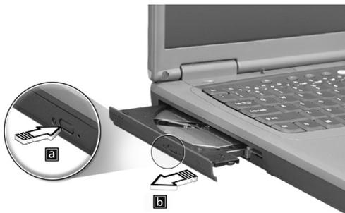
When the power is off, you can eject the drive tray using the emergency eject hole. See page 48.
