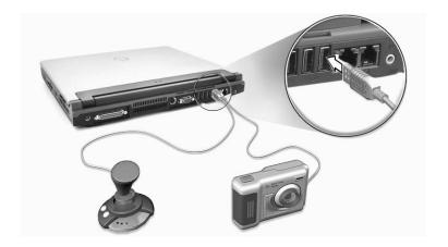
USB is plug and play, which means that you can connect and start using a USB device without having to restart your computer. You can also disconnect the device at any time.
