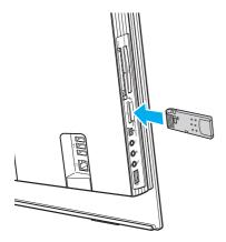
Be sure to hold the Memory Stick media with the arrow pointing in the correct direction as you insert it into the slot. To avoid damaging your computer or the Memory Stick media, do not force the Memory Stick media into the slot if you cannot insert it smoothly.
