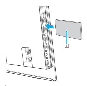
Insert the ExpressCard slot protector to protect against debris entering the slot when not using an ExpressCard module. Before moving your computer, make sure to insert the ExpressCard slot protector into the slot.
