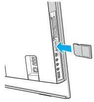
3 Carefully slide the memory card into the slot until it clicks into place. Do not force the card into the slot.
