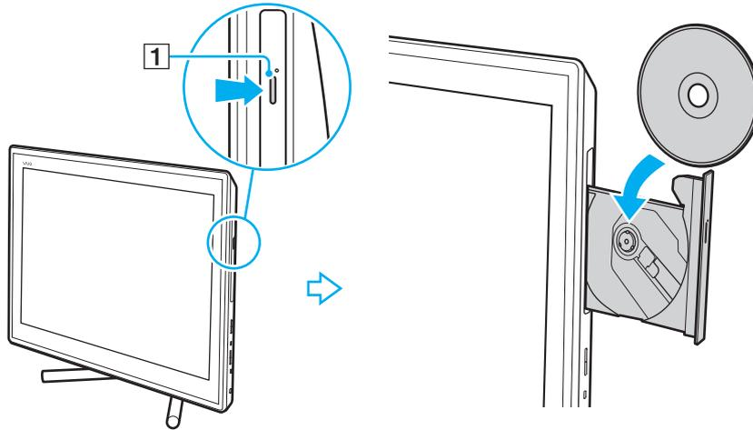
! Do not exert pressure on the drive tray. Be sure to hold the back of the drive tray when placing/removing a disc onto/from the drive tray.
