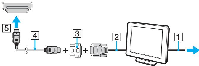
! Your computer is compliant with the HDCP standard and capable of encrypting the transmission channel of digital video signals for the purpose of copyright protection, which enables you to play and view a wide variety of copyright protected and high-quality content. To view the copyright protected content, connect an HDCP-compliant monitor to your computer. If your computer has a non-compliant monitor connected, you will not be able to play or view any copyright protected content.
