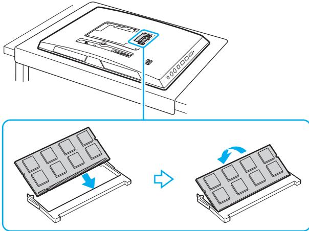
**!** Do not touch any components on the motherboard other than the memory module.
