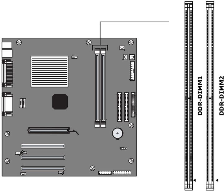
Both sides of each Double-data rate, Dual Inline Memory Module (DDR-DIMM) look very similar. The side with pin 1 has a small "1" to the left of pin 1. Be sure to orient the memory module correctly in the DDR-DIMM slot (a small triangle on the slot indicates pin 1).
