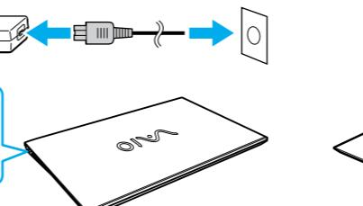
Plug the power cord and the AC adapter into an AC outlet and the computer.
