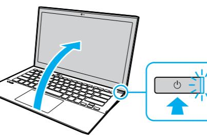
Press and hold down the power button until the power indicator light turns on.
