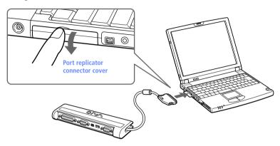
Plug the port replicator cable into the port replicator connector on the computer.
