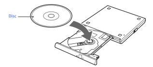
Close the tray by pushing it gently. The BUSY indicator on the drive flashes while your computer is reading data from the disc.
