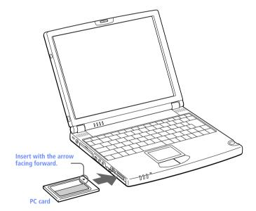
Do not force a card into the slot. It may damage the connector pins.
