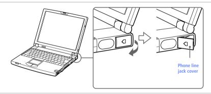
Plug one end of the phone cable (optional) into the jack on the inside of the phone line jack cover. Make sure you insert the phone cable from the rear of the computer and that the modular jack clicks into place.
