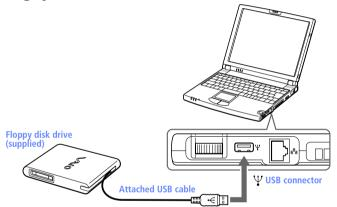
$\triangle$  To use two USB devices at the same time, plug the second device into the  $\Psi$  connector on the left side of the computer, using the supplied conversion adapter.
