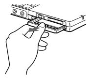
Insert the PC card into the PC card slot, front label facing up. Gently push the card into the slot until the card is fixed into the connector. The release button comes out.
