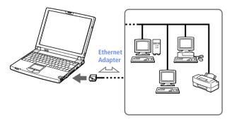
Warning: Only connect 10BASE-T and 100BASE-TX cables to the  $\frac{9}{100}$  (Ethernet network) connector. Do not connect any other type of network cable or any telephone line. Connecting cables other than those listed above may result in an electric current overload and could cause a malfunction, excessive heat, or fire in the connector. To connect the unit to the network, contact your network administrator.
