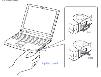
The Jog Dial control window always appears in the display. It is either in the launcher mode or in the guide mode.
