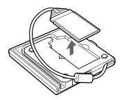
Insert the PC card into the PC card slot with the SONY logo facing up. See "Using PC Cards" on page 32 for details.
