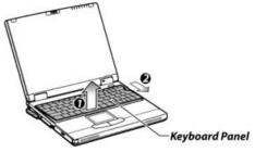
5. To completely release the keyboard panel from the chassis, lift the front of the keyboard panel up about a quarter of an inch. Then slide the keyboard panel forward about a quarter of an inch.
