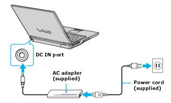
2 Plug the power cord into the AC adapter and an AC outlet.
