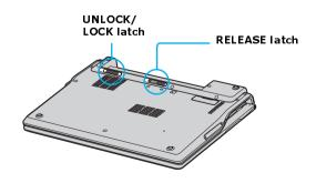
Align the grooves on the battery with the tabs and notches on the back of the computer, and slide the battery toward the computer until it clicks into place.
