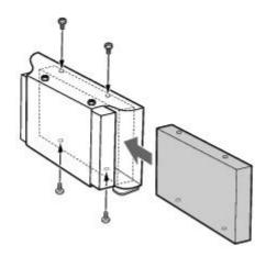
8. Secure the drive to the drive holder with screws, using the two holes on each side of the drive holder.
