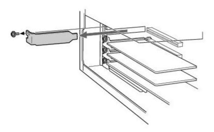
Install the add-on card by inserting it into the expansion slot and securing it with the screw from the expansion slot cover.
