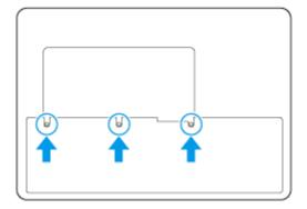
Screws marked by arrows are behind the battery.
