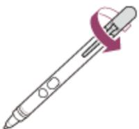
2. Insert the battery into the pen with the + side toward the nib.
