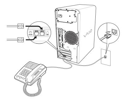
Your computer has a protective sticker is covering the Ethernet port located on the rear panel. Connect only 10BASE-T and 100BASE-TX cables to the Ethernet port. Using other cables or a telephone cable may result in an electric current overload that can cause a malfunction, excessive heat, or fire in the Ethernet port. For help on connecting to a network, see your network administrator.
