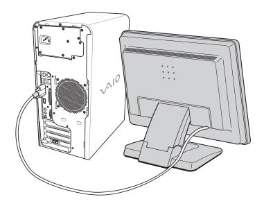
Install your equipment so that you can easily reach the power outlet in the event of an emergency.
