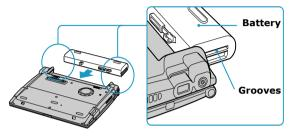
4 Slide the lock lever into the **LOCK** position to secure the battery on the notebook.
