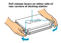
2 Remove the notebook from the docking station, while moving the notebook slightly back to disengage it from the two front latches of the docking station.
