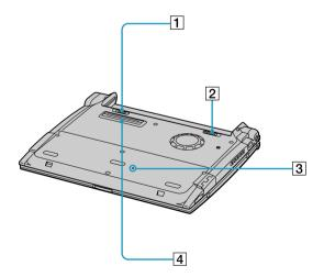
**12** Close the notebook cover, then tighten the screws on the bottom of the computer.
