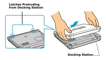
**3** Firmly press down the two rear corners of the notebook until it clicks into place and is securely fastened to the docking station.
