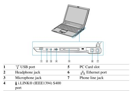
M Only connect 10Base-T and 100Base-TX cables to the <sup>□</sup>/<sub>5</sub> Ethernet port. Do not connect any other type of network cable or any telephone line. Connecting cables other than those listed above may result in an electric current overload and could cause a malfunction, excessive heat, or fire in the port. To connect the unit to the network, contact your network administrator.
