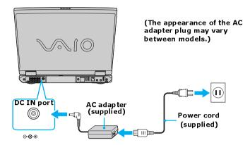
2 Plug one end of the power cord into the AC adapter, and plug the other end into an AC outlet
