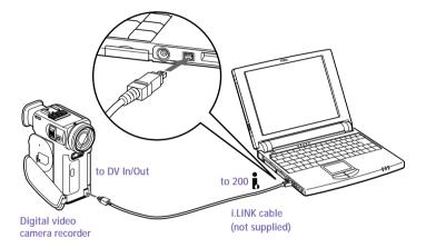
The Sony digital video camera recorder (DCR-PC7) is pictured; your digital video camera recorder may need to be connected differently.
