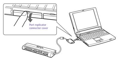
3 Plug the port replicator cable into the port replicator connector on the computer.
