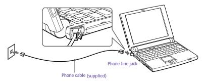
Your computer does not work with party lines, cannot be connected to a coin-operated telephone, and may not work with multiple phone lines or a private branch exchange (PBX). Some of these connections might result in excess electrical current and could cause a malfunction in the internal modem.
