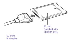
Insert the PC card into the PC card slot with the label side facing up. See "Using PC Cards" on page 26 for details.
