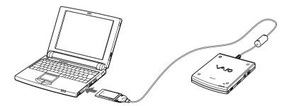
Connect the CD-ROM drive AC power adapter to the CD-ROM drive and plug the AC adapter into an AC outlet.
