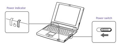
if you hold the power switch in the on position for more than four seconds, the computer turns off.
