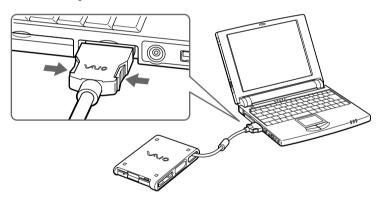
3 Fold the floppy disk drive cable into the compartment on the side of the floppy disk drive.
