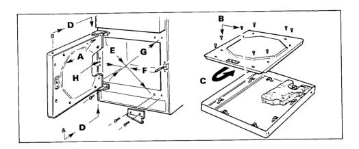
(i) Open door wide and support whilst removing the two screws from the top L.H. hinge bracket. Remove hinge bracket and place to one side. Having done so, the door can now be lifted off the bottom hinge pin (A).
