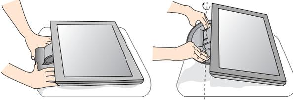
2. Place the monitor with its front facing downward and then further expand the stand base fully to 90 degrees. Do not apply excessive force to expand the stand base over 90 degrees as it may damage the monitor.
