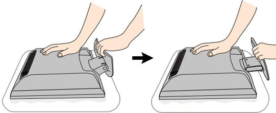
3. Place the monitor upright and adjust the angle of the stand base as desired. Adjust the stand base angle with two hands, holding the monitor head.
