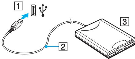
**!** When using a USB floppy disk drive, do not apply force on the USB port. This may cause a malfunction.
