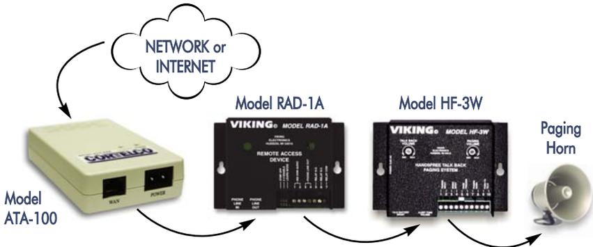
Since the HF-3W is a talkback paging amplifier, the ATA-100 in this case both converts network data to analog paging signal and encodes the talkback signal to data packets that can be sent over the network. If the paging system is analog, another ATA-100 is needed to perform encoding/decoding functions at the originating end.
