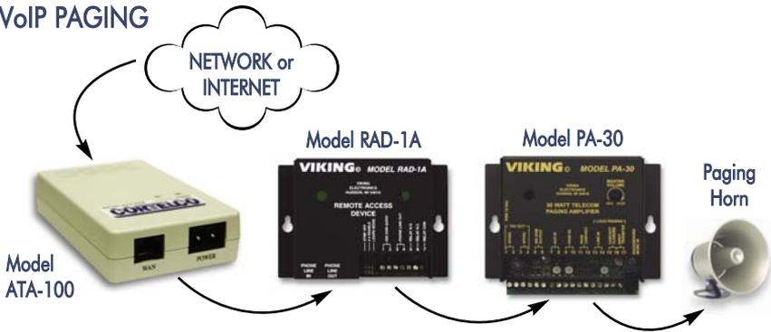
In this example the ATA-100 converts network packets back to an analog paging signal which is amplified by the PA-30 Paging Amplifier. Note that if the paging system is analog, it is necessary to encode the audio paging signal using another ATA-100 before sending it out over the network.
