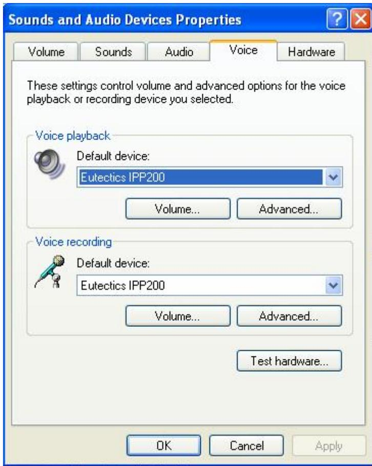
In the Voice tab choose the Eutectics Device (IPP200 in the above example) as the Playback and Recording - also click on the Volume Button and adjust the master volume to the highest level (you can make it lower later if desired).
