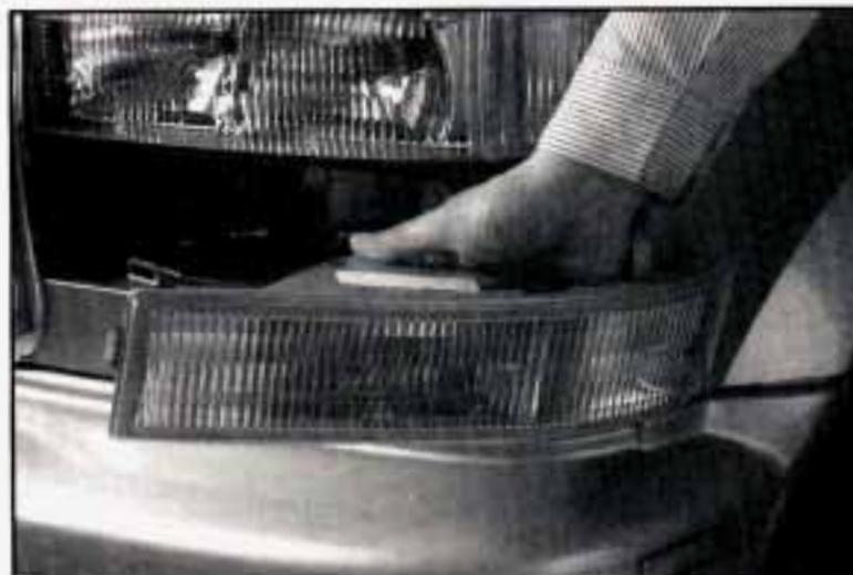
3. Completely remove the sidemarker/turn signal lamp by pulling out the assembly and disconnecting the side marker/turn signal lamp sockets from the lamp.
