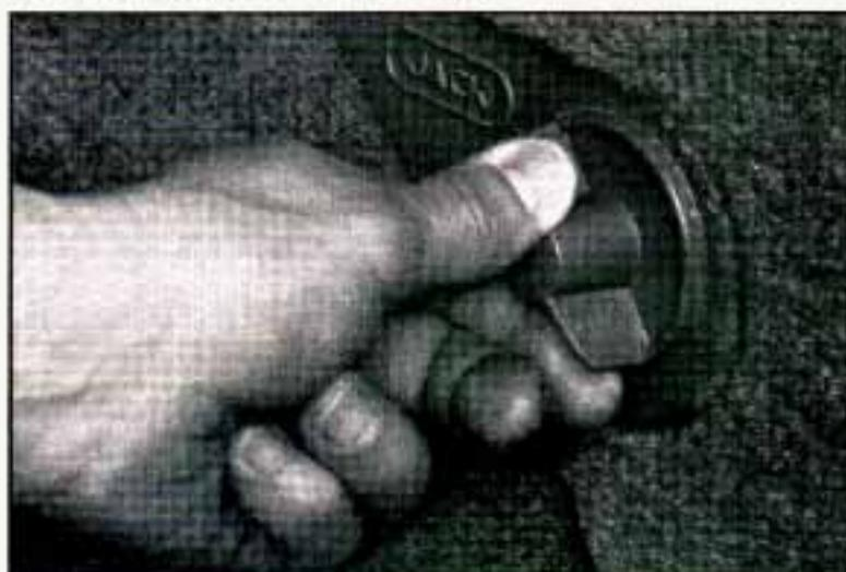
Remove your jack cover by turning the plastic wing nut counterclockwise.
