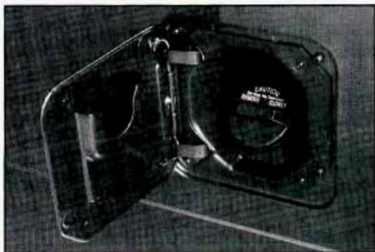
The cap is behind a hinged door on the driver's side of your vehicle.
