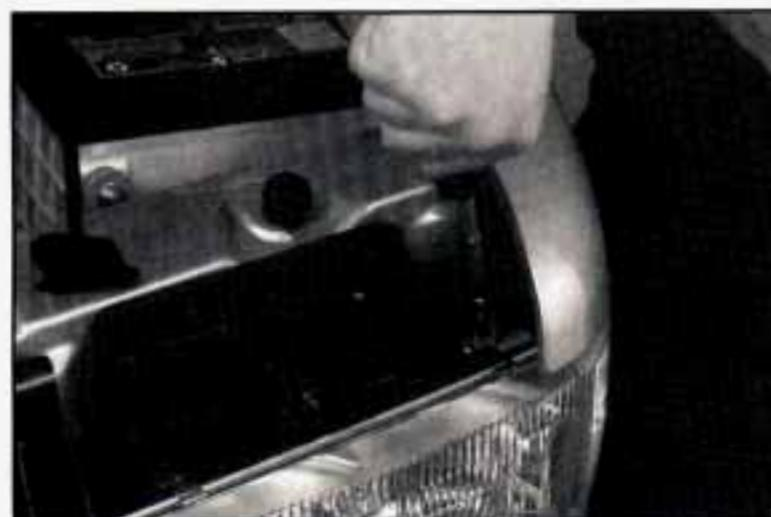
4. Remove the screw located behind the corner reflector in order to remove the entire corner reflector.
