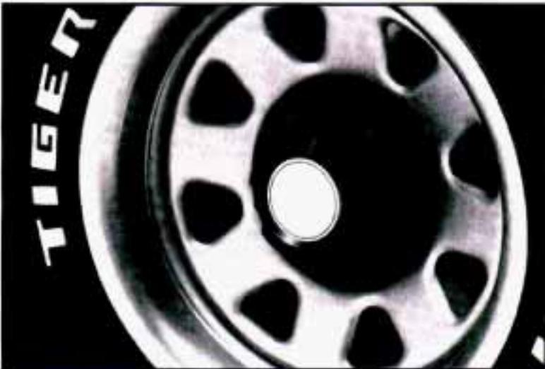
If the wheel has a plastic center cap, you do not have to remove the center cap to loosen the wheel nuts.
