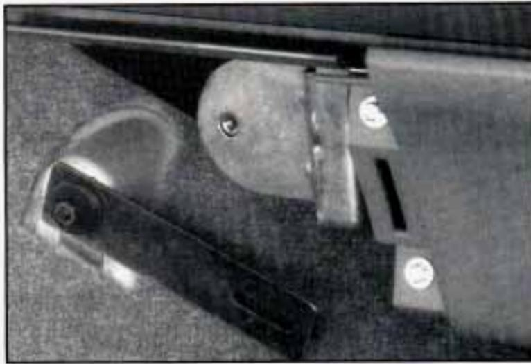
8. Loosen the nut and move the bracket out of the way.
