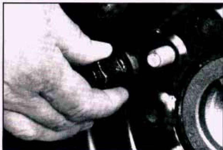
Put on the spare tire. Put the nuts on by hand. Make sure the cone-shaped end is toward the wheel. Tighten each nut by hand until the wheel is held against the hub. If a nut can't be turned by hand, use the extension and see your dealer as soon as possible.
