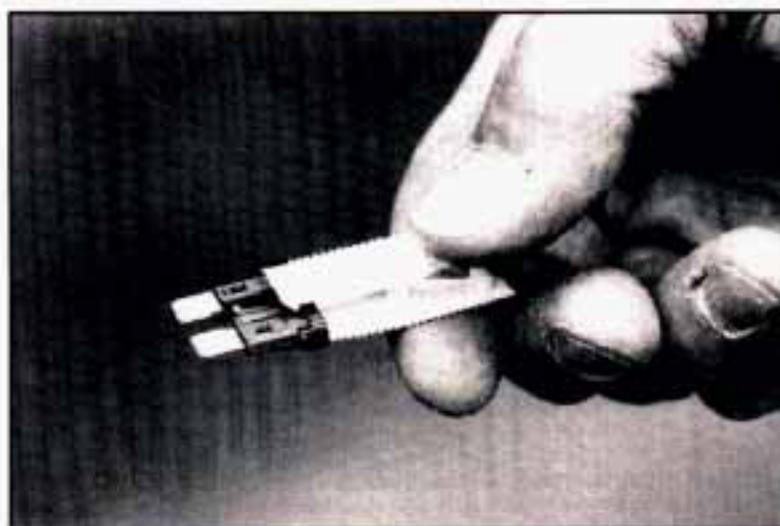
You can remove fuses with a fuse extractor.
