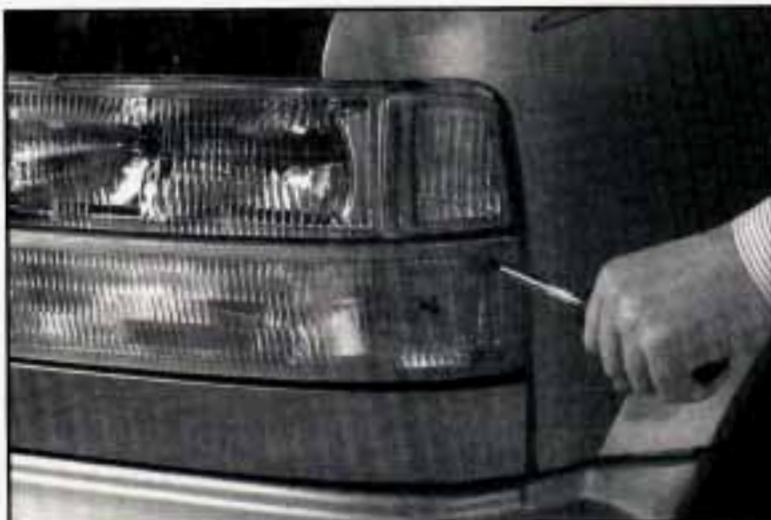
2. Remove the two screws from the side marker/turn signal lamp.
