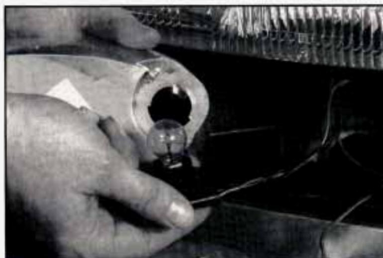
3. Squeeze the tab on the side of the lamp socket while turning the socket counterclockwise.
