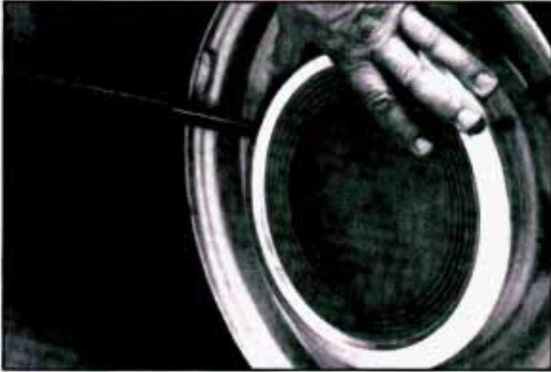
If you have a standard hub cap, remove it by using the flat end of the extension.
