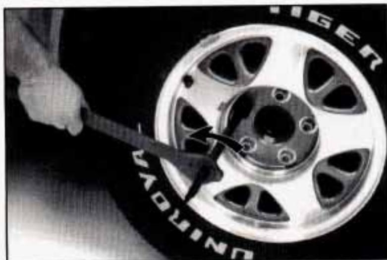
With DOWN facing you, use the ratchet and socket to loosen all the wheel nuts. Don't remove them yet.
