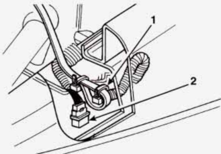
1. Engine Coolant Heater Strap
