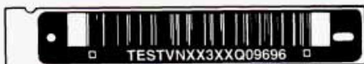
This is the legal identifier for your vehicle. It appears on a plate in the front corner of the instrument panel, on the driver's side. You can see it if you look through the windshield from outside your vehicle. The VIN also appears on the Vehicle Certification and Service Parts labels and the certificates of title and registration.
