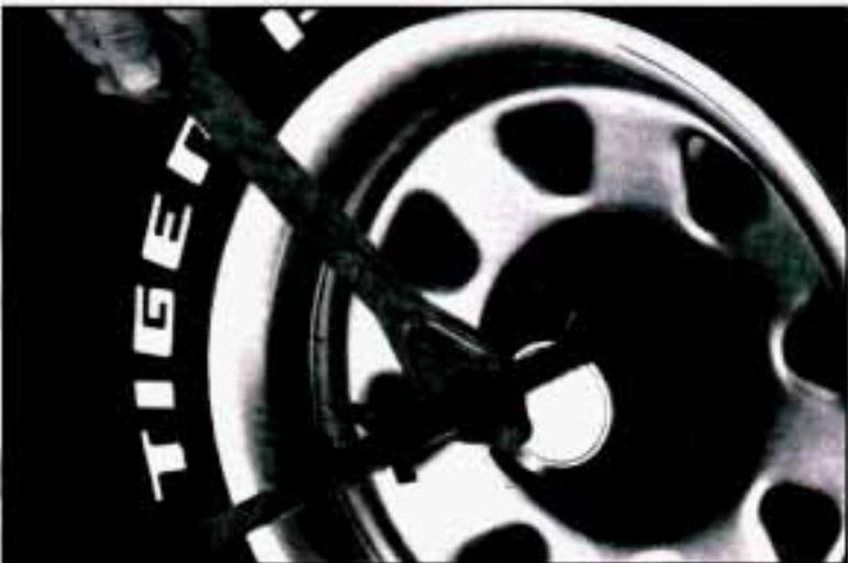
Place the ratchet and socket end of the extension on the wheel nut with the center cap on.
