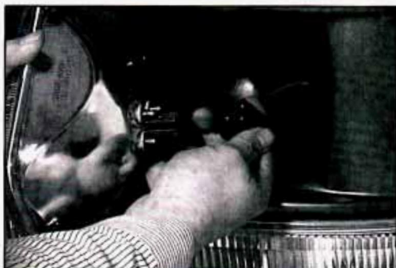
5. Pull the connector out and unplug the lamp.
