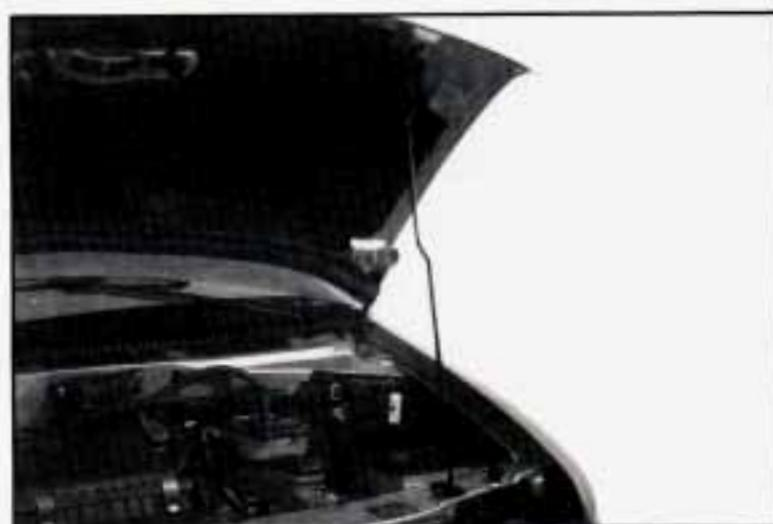
Before closing the hood, be sure all the filler caps are on properly. Then lift the hood to relieve pressure on the hood prop.
