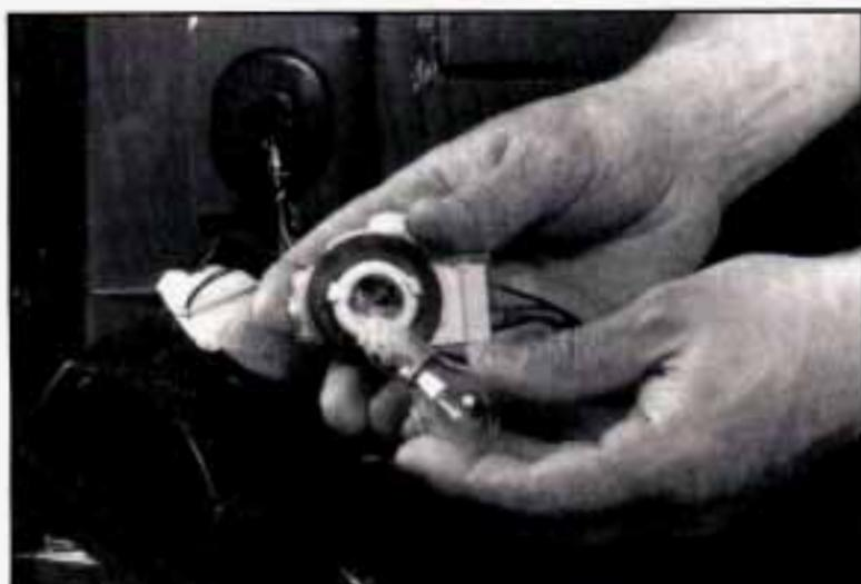
5. Pull out the bulb and replace it with the new bulb.
