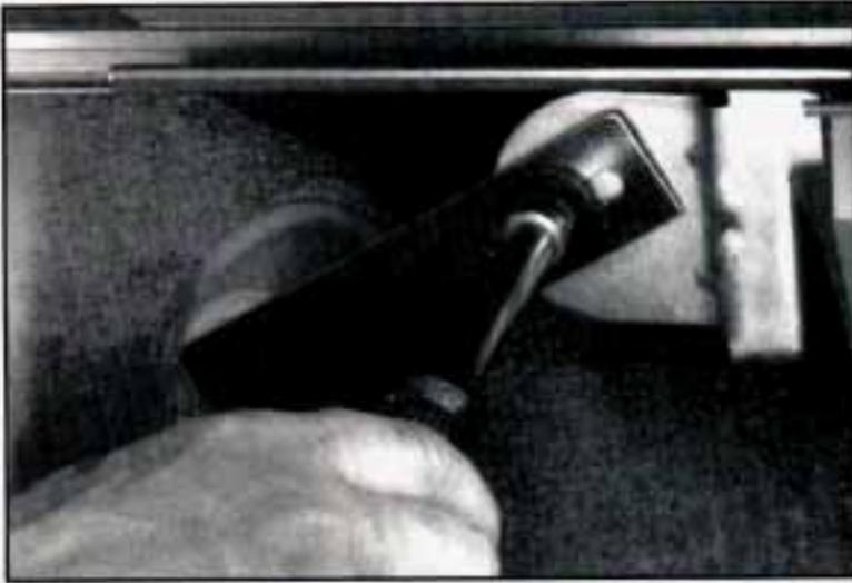
7. Remove the bolt from the engine cover bracket.
