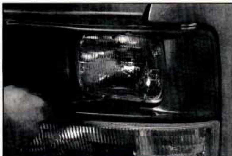
2. Remove the four screws from the headlamp bezel. Pull the bezel out so you can see the parking/turn signal sockets.
