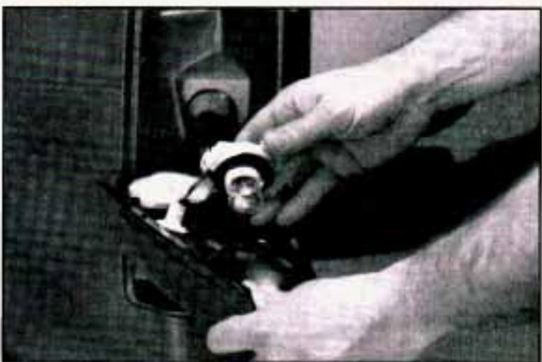
4. Press the tab and turn the socket counterclockwise to remove the socket from the bezel. If the socket does not have a tab, turn the socket counterclockwise to remove the socket from the bezel.
