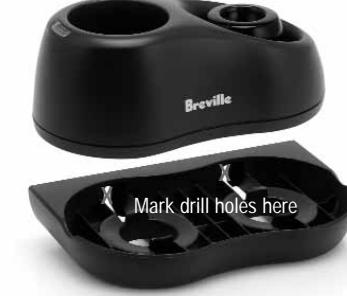
3. Drill a 0.2inch (5mm) diameter hole through the center of each drill hole mark. Push a plastic wall anchor into each drilled hole.
