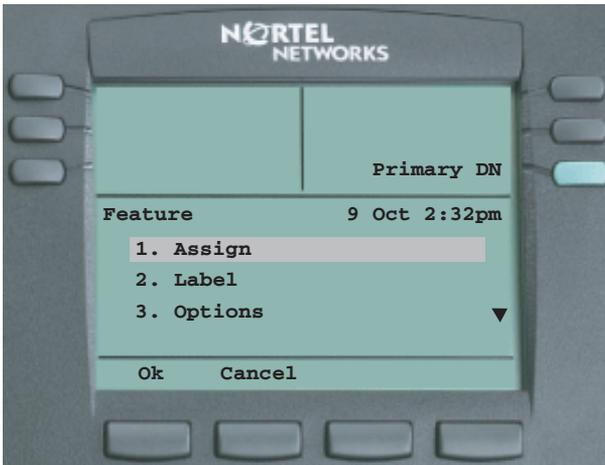
2. Scroll through the Assign menu using the navigation keys so that Key Type appears (the first item in the list) and press **Ok** or press **Cancel** to return to the Feature menu.
