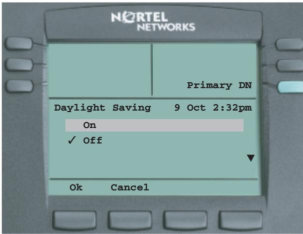
The "✓" in front of the time zone indicates your current selection (that is, Daylight Savings disabled). Press **Ok** to turn off Daylight Savings or press **Cancel** to return to the Time menu.
