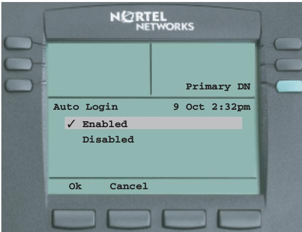
You can toggle between enabling the Auto Login functionality by pressing the down navigation key. Press **Ok** to save the setting and return to the User menu. Press **Cancel** to return to the User menu without saving your changes.
