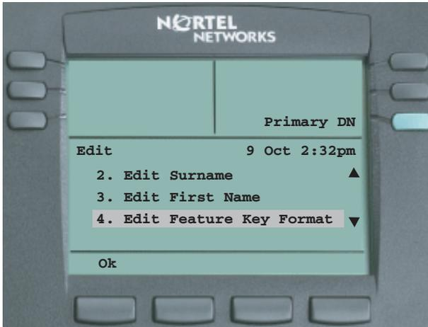
6. Edit the feature key on which you want the entry to appear, if required, and press **Ok** (if you do not want the entry to appear on a feature key, press **Ok** without making an entry). The following screen appears:
