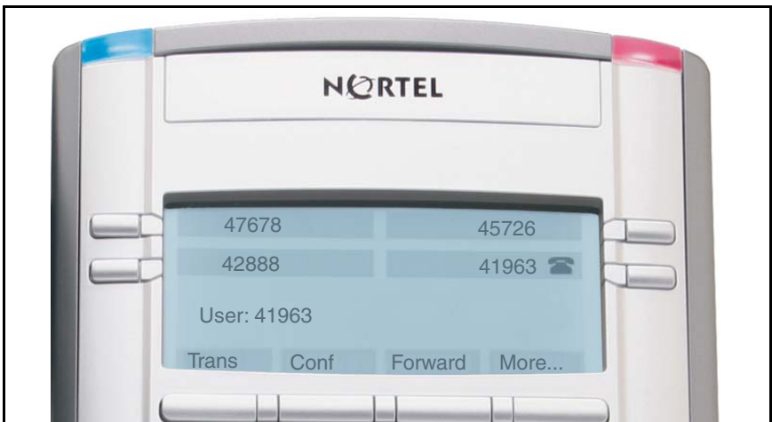
Figure 10: Logged in to an IP Phone 1140E using an IP Phone 1120E
