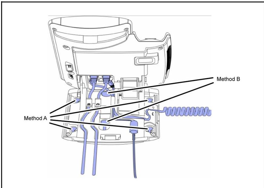
8. Wall-mount your phone (optional). Your IP Phone 1120E can be mounted either by: (Method A) using the mounting holes on the bottom of the phone stand, or (Method B) using a traditional-style wall-mount box with an RJ-45 connector and a 15-cm (6-inch) RJ-45 cord (not provided).
