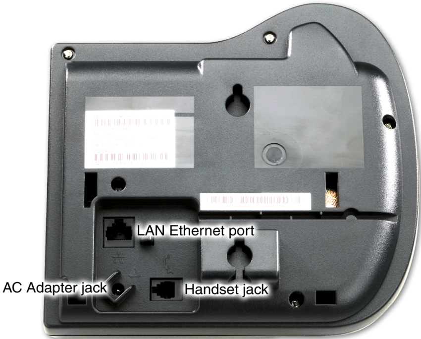
Figure 3: IP Phone 2001 connections
