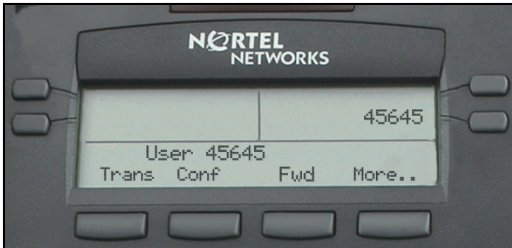
Figure 5: Logged on to an IP Phone 2001 using an IP Phone 2002
