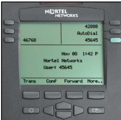
**Figure 7: Logged on to an IP Phone 2002 using an IP Softphone 2050.**
