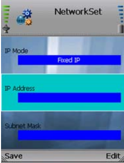
Figure 4-18: Network Settings - Fixed IP
